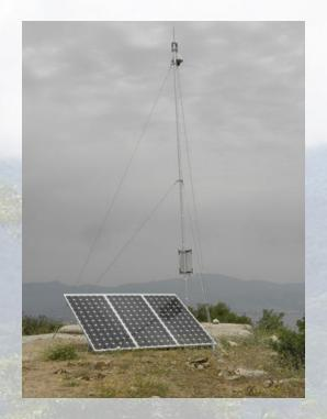
The station responsible for fire and smoke detection is an autonomous unit that continuously operates scanning predefined forest areas. When an event occurs the station communicates with main server and notifies the control center by mail or SMS.
